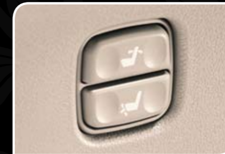
4-way power seat button for desired seating position on second row seat. (2.4 G and 3.5 G)
