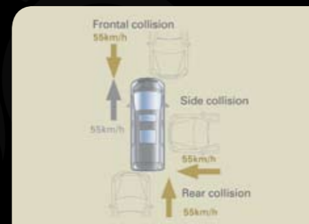
Omni-Directional Compatibility Body Structure
